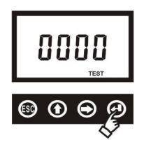
In this mode, the controller switches capacitors on and off one by one in cycle, alternatively for 5 seconds. Each capacitor will follow the rule of Waiting Time (i.e. 180 seconds) before switching on again.
