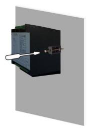
3. Turn the Screw in the Mounting Bracket and tight it.
